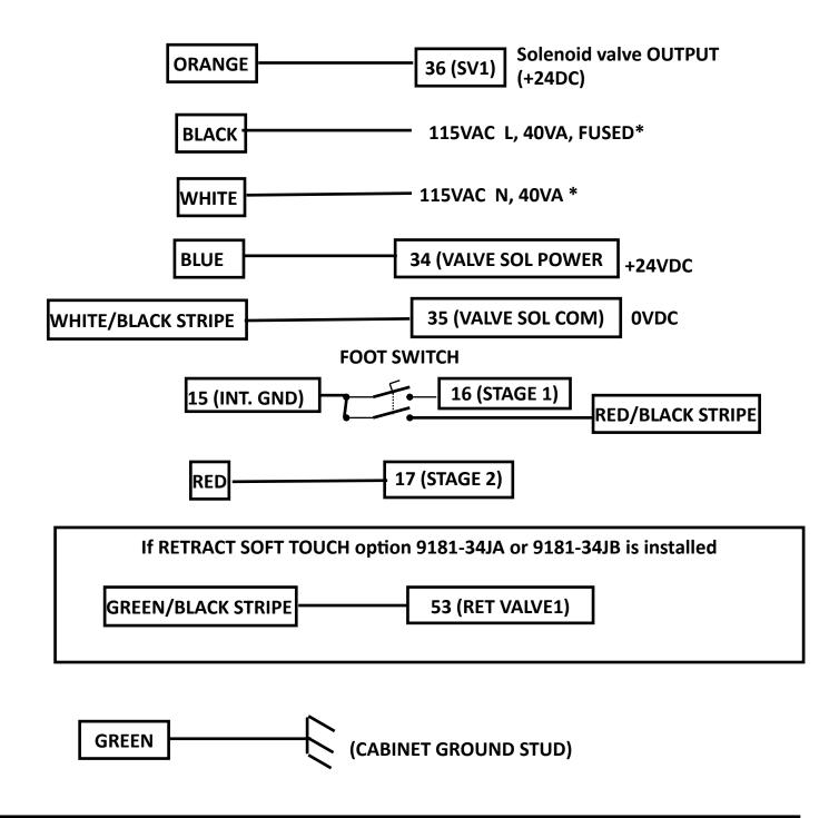
\* If option 9181-34/115 is installed in this unit, the 115V transformer and fuses will already be installed at the factory.
